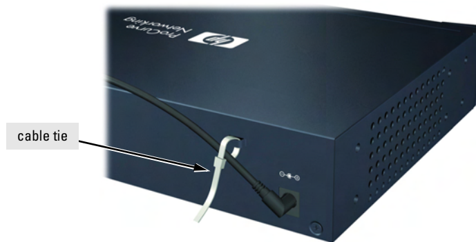
Figure 2-12. Securing the power cord on the Switch 2520G-8-PoE
